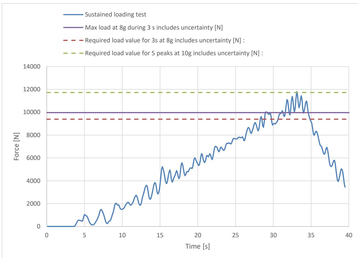
**Sustained loading test results <sup>(3)</sup>**
